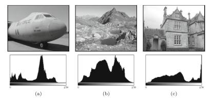
high-value peaks (Fig. 3.6) is representative of an improperly exposed image.
