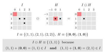
Fig. 9.9 Binary erosion example. The binary image I is subject to erosion with H as the structuring element. H is only covered by I when placed at position p = (1, 1), thus the resulting points set contains only the single coordinate (1, 1).
