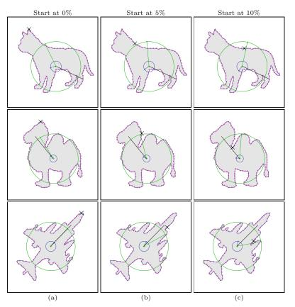
In particular, we see from Eqn. (26.90) that shifting the start position modifies the coefficients of the *first* descriptor pair  $FP_1 = (G_{-1}, G_{+1})$  to
