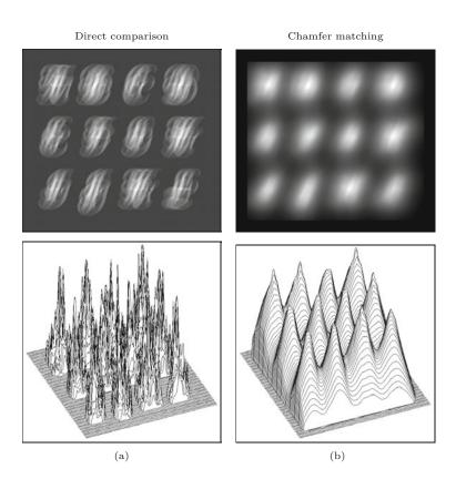
the method is based on minimizing the distances to foreground pixels. One way to reduce the probability of false matches is not to use a *linear* summation (as in Eqn. (23.25)) but add up the *squared* distances, that is,
