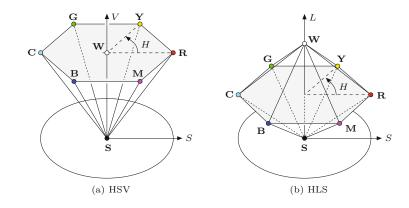
on the bottom tip and white on the top. The primary colors lie on the corner points of the hexagonal base between the two pyramids. Even though it is often portrayed in this intuitive way, mathematically the HLS space is again a cylinder (see Fig. 12.15).
