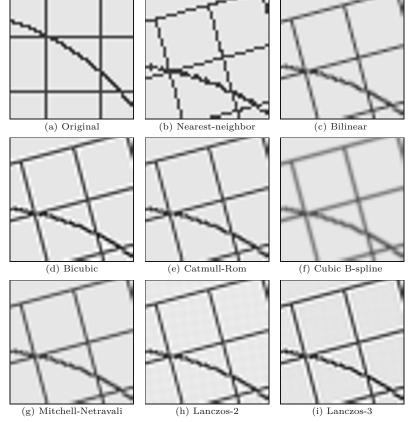
Fig. 22.22 Image interpolation methods compared (line art).
