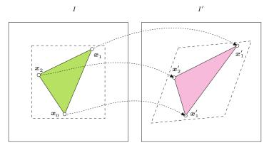
six transformation parameters  $a_{00}, \ldots, a_{12}$  are derived by solving the system of linear equations
