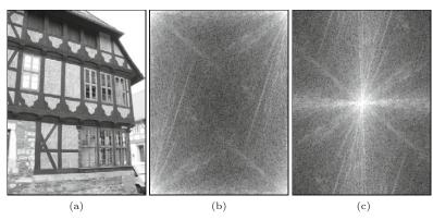
respectively. This can be easily accomplished by swapping the four quadrants of the Fourier transform, as illustrated in Fig. 19.3. In the resulting representation, the low-frequency coefficients are found at the center and the high-frequency entries along the outer boundaries. Figure 19.4 shows the plot of a 2D power spectrum as an intensity image in its original and centered form, with the intensity proportional to the logarithm of the spectral values  $(\log_{10} |G(m, n)|)$ .
