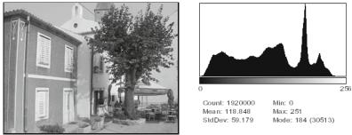
The histogram h for a grayscale image I with intensity values in the range  $I(u, v) \in [0, K-1]$  holds exactly K entries, where  $K = 2^8 =$ 256 for a typical 8-bit grayscale image. Each single histogram entry is defined as
