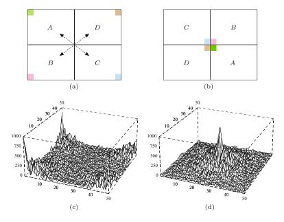
Fig. 19.4 Intensity plot of a 2D power spectrum: original image (a), noncentered spectrum (b), and centered spectrum (c).
