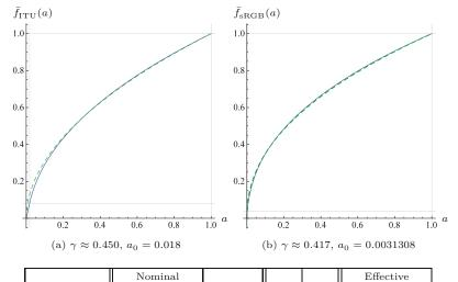
Table 4.1 Gamma correction parameters for the ITU and sRGB standards based on the modified mapping in Eqns. (4.34) and (4.35).
