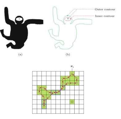
to *first* identify the connected regions in the image and *second*, for each region, proceed around it, starting from a pixel selected from its border. In the same way, an internal contour can be found by starting at a border pixel of a region's hole. A wide range of algorithms based on first finding the regions and then following along their contours have been published, including [202], [180, pp. 142–148], and [214, p. 296].
