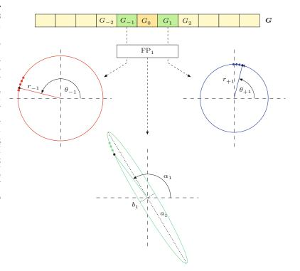
Like its constituting circles, this ellipse is centered at  $(x_c, y_c) = (0, 0)$ and performs *m* revolutions for one traversal of the contour.  $G_{-m}$ specifies the circle
