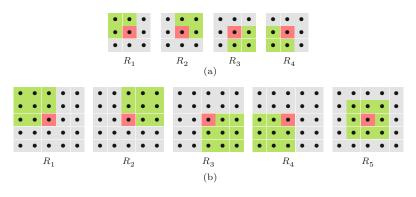
Note that replacing a pixel value by the mean of a square neighborhood is equivalent to linear filtering with a simple box kernel, which is not an optimal smoothing operator. To reduce the artifacts caused by the square subregions, alternative filter structures have been proposed, such as the  $5 \times 5$  Nagao-Matsuyama filter [170] shown in Fig. 17.2.
