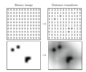
the image twice by propagating the computed values across the image like a wave. The first traversal starts at the upper left corner of the image and propagates the distance values downward in a diagonal direction. The second traversal proceeds in the opposite direction from the bottom to the top. For each traversal, a "distance mask" is used for the propagation of the distance values; that is,
