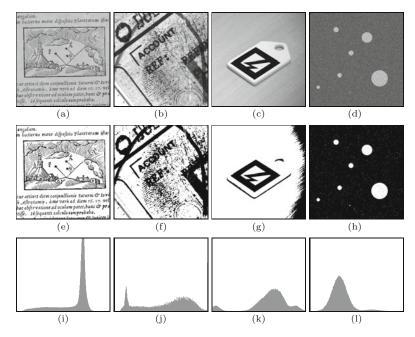
of the *background* or the *foreground*. Thus the set of all image pixels is partitioned into two disjoint sets  $C_0$  and  $C_1$ , where  $C_0$  contains all elements with values in  $[0, 1, \ldots, q]$  and  $C_1$  collects the remaining elements with values in  $[q+1, \ldots, K-1]$ , that is,
