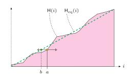
The desired point operation  $f_{eq}()$  is simply obtained from the cumulative histogram H of the original image as<sup>4</sup>
