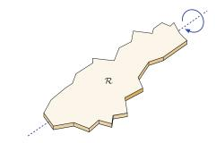
the pencil exhibits the least mass inertia (Fig. 10.17). As long as a region exhibits an orientation at all  $(\mu_{20}(\mathcal{R}) \neq \mu_{02}(\mathcal{R}))$ , the direction  $\theta_{\mathcal{R}}$  of the major axis can be found directly from the central moments  $\mu_{pq}$  as
