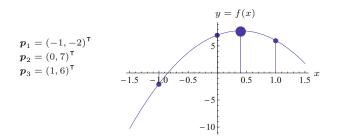
Fig. C.2 Fitting a quadratic function to three reference points at positions  $x_1 = -1, x_2 = 0, x_3 =$ +1. The interpolated, continuous curve has a maximum at
