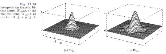
Fig. 22.18 2D interpolation kernels. bilinear kernel  $W_{\text{bil}}(x, y)$  (a) and bicubic kernel  $W_{\text{bic}}(x, y)$
