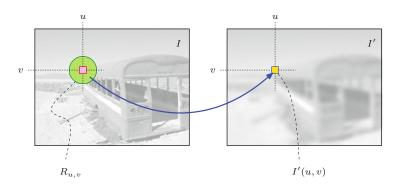
Fig. 5.2 Principal filter operation. Each new pixel value I'(u, v) is calculated as a function of the pixel values within a specified region of source pixels  $R_{u,v}$  in the original image I.
