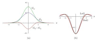
The factor  $\lambda \in \mathbb{R}$  in Eqn. (25.12) controls the magnitude of the DoG function; it depends on both the ratio  $\kappa$  and the scale parameter  $\sigma$ . To match the magnitude of the original LoG (Eqn. (25.6)) at the origin, it must be set to
