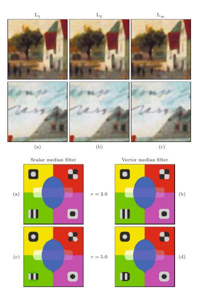
be done in  $\mathcal{O}(n)$ . Since *n* is proportional to the square of the filter radius *r*, the number of steps required for calculating a single image pixel is roughly  $\mathcal{O}(r^4)$ . While faster implementations have been proposed [10, 18, 221], calculating the vector median filter remains computationally demanding.
