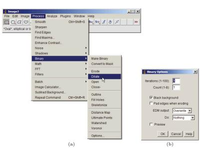
instead, since they provide explicit control of the background pixel value and are thus independent from other settings. ImageJ's Byte-Processor class defines additional methods for morphological operations on binary images, such as outline() and skeletonize(). The method outline() implements the extraction of region boundaries using an 8-neighborhood structuring element, as described in Sec. 9.2.7. The method skeletonize(), on the other hand, implements a thinning process similar to Alg. 9.3.
