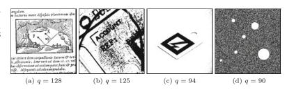
histogram. Figure 11.3 shows the results of thresholding with the isodata algorithm applied to the test images in Fig. 11.1.
