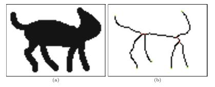
shape representation (see Fig. 9.30 for an example). Use ImageJ's skeletonize() method or the thin() methode of class Binary-MorphologyFilter (see Sec. 9.4.3) to generate the skeleton, then locate and mark the connecting and terminal nodes of this structure. Define precisely the properties of each type of node and use this definition in your implementation. Test your implementation on different examples. How would you generally judge the robustness of this approach as a 2D shape representation?
