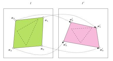
21.3) and the distance ratios between points on a line are not preserved. The projective mapping is therefore sometimes referred to as "perspective" or "pseudo-perspective".
