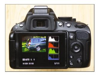
Fig. 3.1 Digital camera back display showing the associated RGB histograms. 3 HISTOGRAMS AND IMAGE STATISTICS
