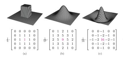
center. The Gaussian filter is isotropic if the discrete filter matrix is large enough for a sufficient approximation (at least  $5 \times 5$ ). As a low-pass filter, the Gaussian is "well-behaved" in frequency space and thus clearly superior to the box filter. The 2D Gaussian filter is separable into a pair of 1D filters (see Sec. 5.3.3), which facilitates its efficient implementation.<sup>2</sup>
