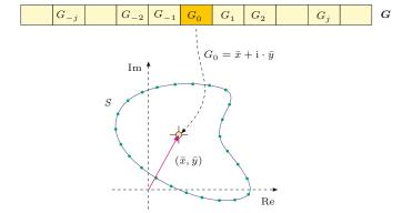
Fig. 26.5 DFT coefficient  $G_0$  corresponds to the centroid of the contour points.
