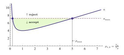
case c is likely to be a good reference point that can be located reliably. In the optimal situation (e.g., near a corner), the ratio of the eigenvalues  $\rho = \lambda_1/\lambda_2$  is close to 1. Alternatively, if the ratio  $\rho$  is high it can be concluded that a single orientation dominates at this position, as is typically the case in the neighborhood of edges.
