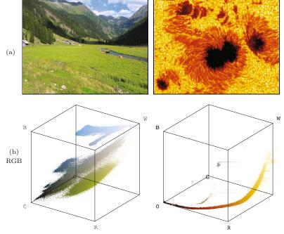
Figure 12.9 shows the distribution of the colors from natural images in the RGB color space. The first half of this section introduces alternative color spaces and the methods of converting between them, and later discusses the choices that need to be made to correctly convert a color image to grayscale. In addition to the classical color systems most widely used in programming, precise reference systems, such as the CIEXYZ color space, gain increasing importance in practical color processing.
