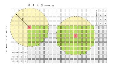
type, however, are not well suited for image smoothing, because they create strong ringing and truncating effects, as demonstrated in Fig. 11.15. Moreover, convolution with a box-shaped (rectangular) kernel is a non-isotropic operation, that is, the results are orientation-dependent. From this perspective alone it seems appropriate to consider other smoothing kernels, Gaussian kernels in particular.
