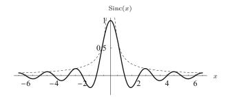
Fig. 22.3 Sinc function in 1D. The function Sinc(x) has the value 1 at the origin and zero values at all integer positions. The dashed line plots the amplitude  $|\frac{1}{\pi x}|$  of the underlying sine function.
