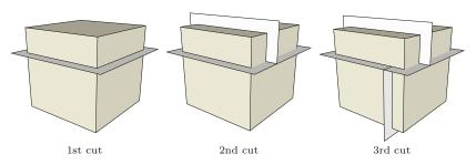
The result of this recursive splitting process is a partitioning of the color space into a set of disjoint boxes, with each box ideally containing the same number of image pixels. In the last step, a representative color vector (e.g., the mean vector of the contained colors) is computed for each color cube, and all the image pixels it contains are replaced by that color.
