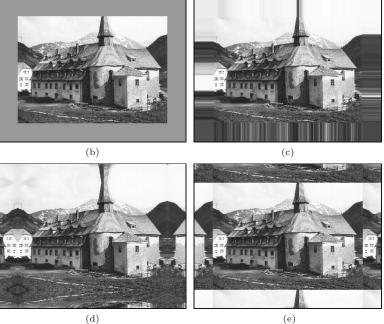
None of these methods is perfect and, as usual, the right choice depends upon the type of image and the filter applied. Notice also that the special treatment of the image borders may sometimes require more programming effort (and computing time) than the processing of the interior image.
