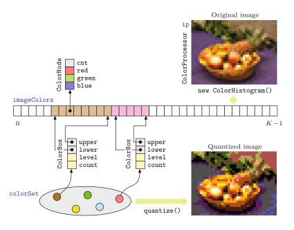
**Exercise 13.2.** The median-cut algorithm for color quantization (Sec. 13.2.2) is implemented in the *Independent JPEG Group's*<sup>4</sup> **libjpeg** open source software with the following modification: the choice of the cube to be split next depends alternately on (a) the number of contained image pixels and (b) the cube's geometric volume. Consider the possible motives and discuss examples where this approach may offer an improvement over the original algorithm.
