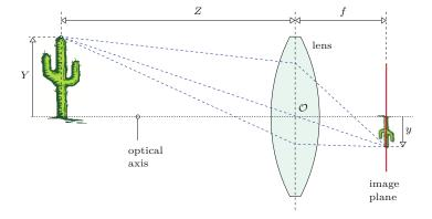
Fig. 1.3 Thin lens projection model.
