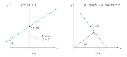
as the reference point for the x/y image coordinates, then it is possible to limit the range of the radius to half the diagonal of the image, that is,
