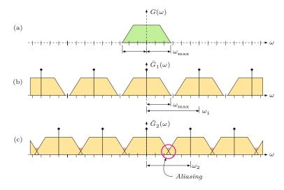
As a consequence, the spectrum  $G(\omega)$  of the original continuous signal becomes *replicated* in the Fourier spectrum  $\bar{G}(\omega)$  of a sampled signal at every pulse of the sampling function's spectrum; that is, infinitely many times (see Fig. 18.8(a, b))! Thus the resulting Fourier spectrum is repetitive with a period  $\frac{2\pi}{\tau}$ , which corresponds to the sampling frequency  $\omega_s$ .
