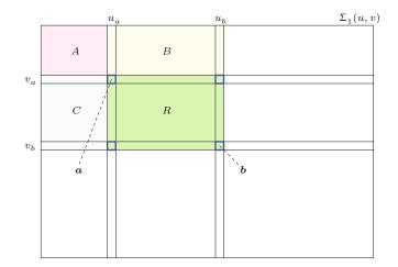
Thus a value in  $\Sigma_1$  is the sum of all pixel values in the original image I located to the left and above the given position (u, v), inclusively. The integral image can be calculated efficiently with a single pass over the image I by using the recurrence relation
