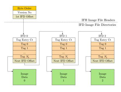
so that it is possible, for example, to store a number of variations of an image in different sizes and representations together in a single TIFF file. The flexibility of TIFF has made it an almost universal exchange format that is widely used in archiving documents, scientific applications, digital photography, and digital video production.
