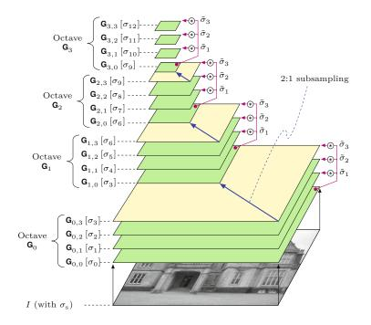
From the octave's base level  $\mathbf{G}_{p,0}$ , the subsequent levels in the same octave can be calculated by filtering with relatively small Gaussian kernels. The size of the kernel needed to calculate scale-level  $\mathbf{G}_{p,q}$  from the octave's base level  $\mathbf{G}_{p,0}$  is obtained from the corresponding decimated scales (Eqn. (25.37)) as
