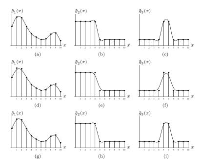
22.12(g–i) show that this method is a good compromise, creating little overshoot, high edge sharpness, and good signal continuity in smooth regions. Since the resulting function does not pass through the original sample points, the Mitchell-Netravali method is again an *approximation* and not an interpolation.
