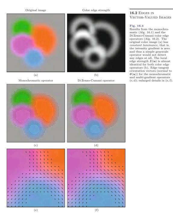
maximum edge strength  $\sqrt{\lambda_1(\boldsymbol{u})} = \|\nabla I(\boldsymbol{u})\|_2$  is equivalent to the magnitude of the local intensity gradient.<sup>13</sup> The fact that  $\lambda_2 = 0$  indicates that the local contrast in the orthogonal direction (i.e., along the edge tangent) is zero (see Fig. 16.3(c)).
