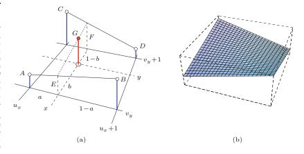
where  $u_x = \lfloor x \rfloor$  and  $v_x = \lfloor y \rfloor$ . Then the pixel values A, B, C, D are interpolated in horizontal and subsequently in vertical direction. The intermediate values E, F are calculated from the distance  $a = (x - u_x)$ of the specified interpolation position (x, y) from the discrete raster coordinate  $u_x$  as
