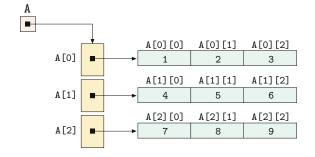
then A is actually a 1D array with three elements, each of which is again a 1D array. The elements A[0], A[1] and A[2] are of type int[] and correspond to the three rows of the matrix A (see Fig. F.1).
