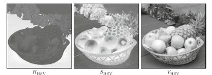
Fig. 12.13 HSV components for the test image in Fig. 12.2. The darker areas in the  $h_{\rm HSV}$  component correspond to the red and yellow colors, where the hue angle is near zero.
