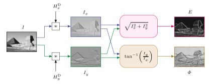
The estimate of the edge orientation based on the original Prewitt and Sobel filters is relatively inaccurate, and improved versions of the Sobel filters were proposed in [126, p. 353] to minimize the orientation errors:
