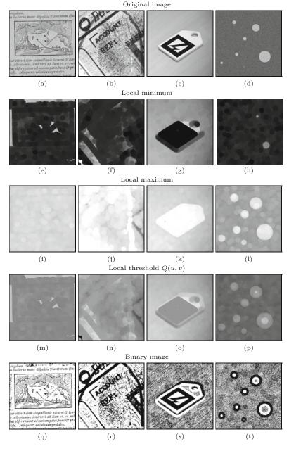
of the background. A size of  $31 \times 31$  pixels (or radius r = 15) is suggested in [172] and  $\kappa = 0.18$ , though the latter does not seem to be critical.
