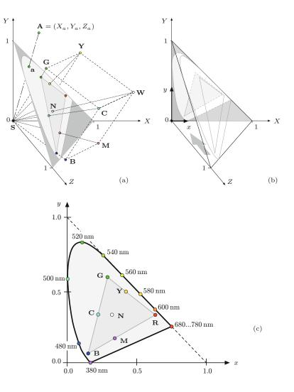
with the same hue but different brightness corresponds to a single x, y point. All possible composite colors lie inside the convex hull specified by the coordinates of the primary colors of the CIE diagram and, in particular, complementary colors are located on straight lines that run diagonally through the white point.
