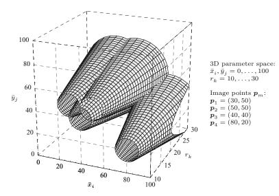
in photographs. While the Hough transform can still be used to find ellipses, the larger parameter space required makes it substantially more expensive.
