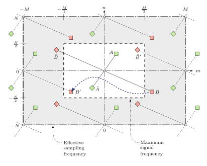
*outside* these limits is reflected across the boundary of this box toward the coordinate center onto lower frequencies, which would appear as visual aliasing in the reconstructed image.
